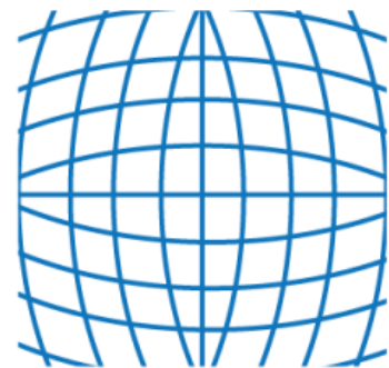
positive radial distortion "barrel"
